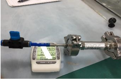
Figure 3. The leak is connected to the hose
