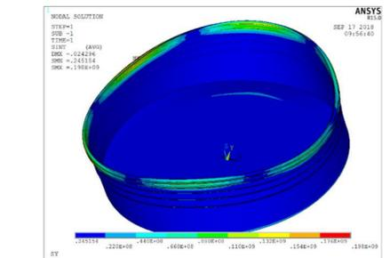
Figure 3. Contour map of stress intensity distribution at a water level of 70cm.
