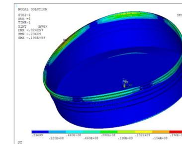
Figure 2. Contour map of stress intensity distribution at a water level of 30cm.
