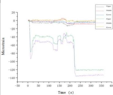
Figure 1. Strain values of sensors at measurement points 3 and 4 at a water level of 30cm
