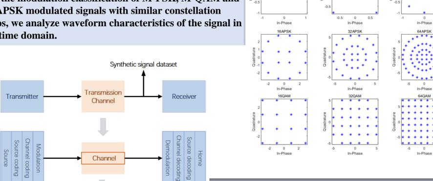
The experimental dataset is generated through the simulation signal transmission process. Then, I/O data in the form of 2\*1024 are obtained.
