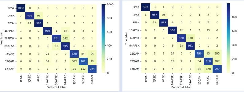
In this paper, the modulation classification method of communication signal based on CNN is proposed. The CNN network directly extracts the features of the original data sequence for classification without manual feature selection.
