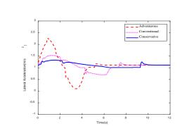
The optimal trajectory under different driving styles is tracked by MPC control, and the lane changing trajectory output by Carsim and the lateral acceleration of the vehicle are collected.
